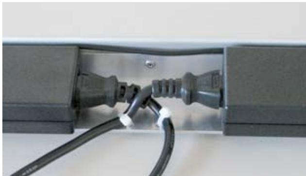
Figure 4-4 Power cable strain relief (with optional redundant power supply)
