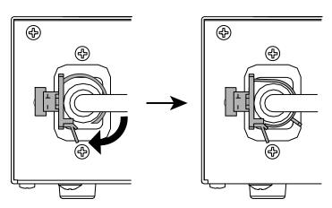
\*Check that the power cord holder is secured.
