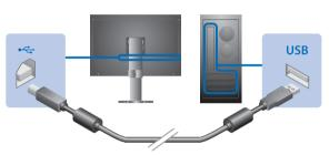
**2** Connect the measurement device to the USB downstream port of the computer or the monitor
