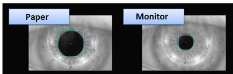
Fig. 25: Comparison of pupil diameter when gazing characters on the paper and screen, in dark environmental illuminances (250 [lx]) and bright screen (270 [cd/m 2 ]).
