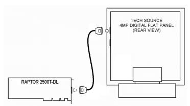
Figure 2-1 – Raptor 2100 Digital Flat Panel Subsystem
