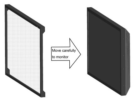
3. Insert the screws which are delivered with the protective screen and fasten the screws. **Notice:** The maximum torque for fastening the screws is 1.6 Nm.
