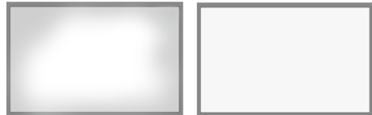
Without DUE: uneven brightness distribution
